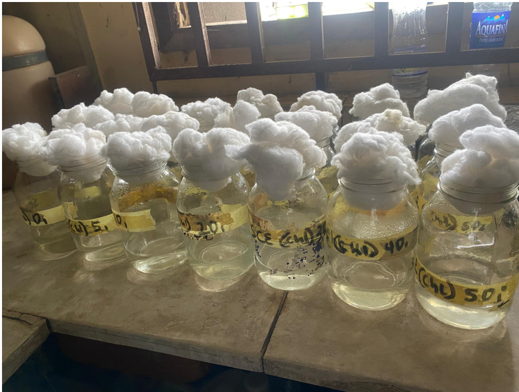
Plate 2: Culture vessels with varying concentrations of the antibiotics (Tetracycline and Chloramphenicol) and the microalga ( Acutodesmus acutiformis ).
