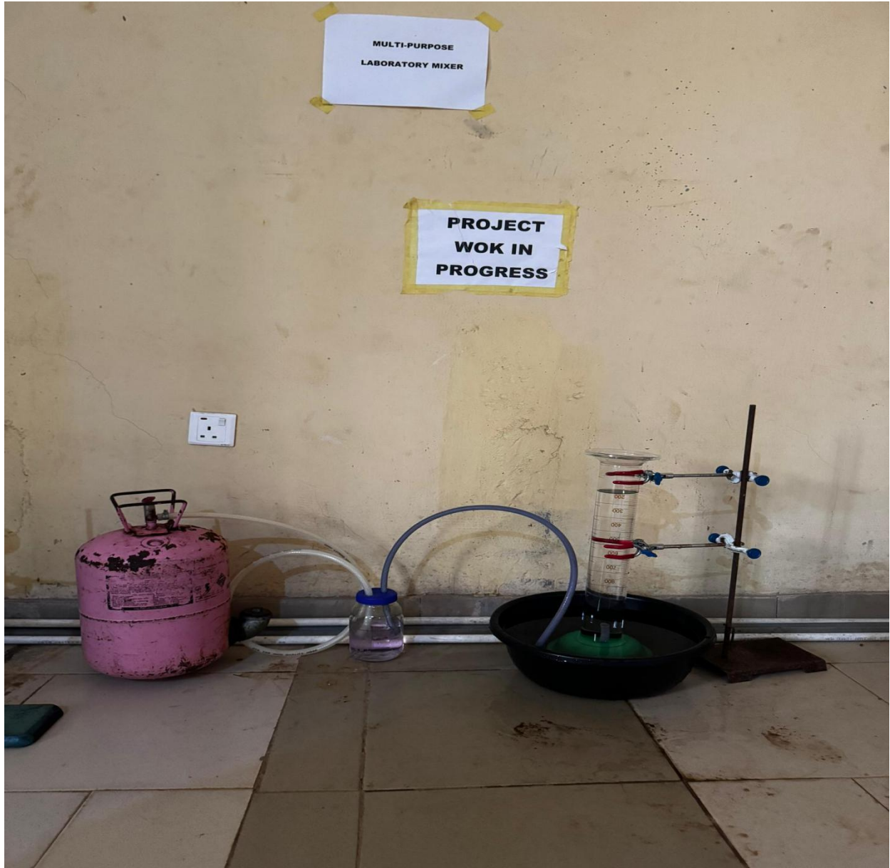
Plate 3.1: Experimental Set up for the Anaerobic Digestion of Cold Digestion of Cattle Rumen Content and Water Hyacinth using Water Displacement Method
