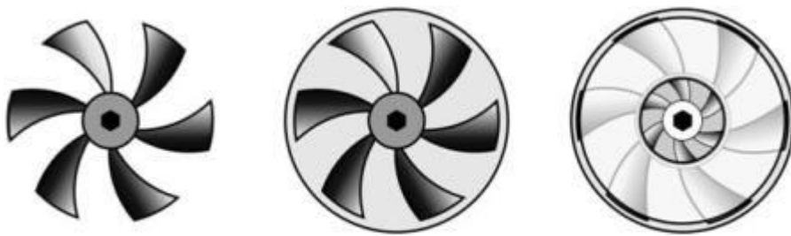
Fig 2.7 - Open, Semi Enclosed and Enclosed Impeller
