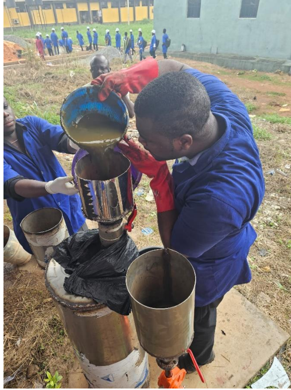
Figure 4.13: Addition of Slurry into Canister
