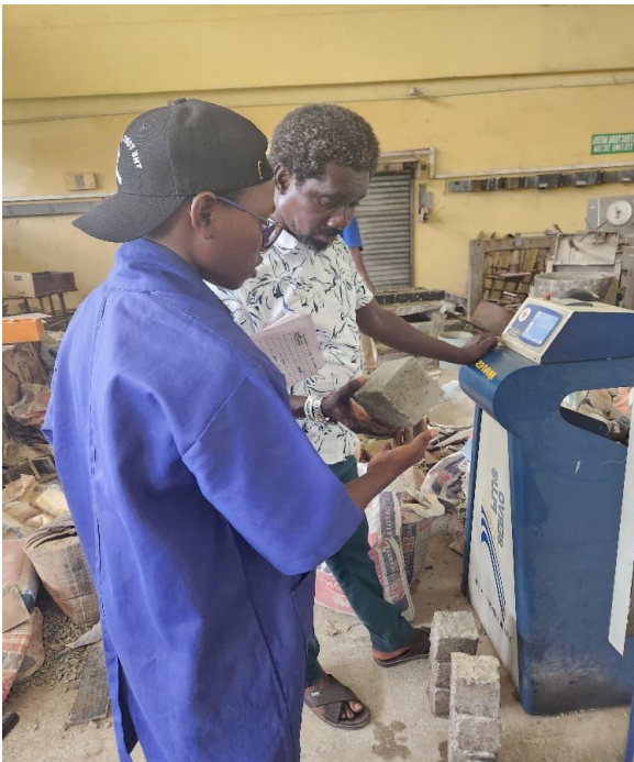
Plate A5: Crushing of Cube During Compressive Strength Test
