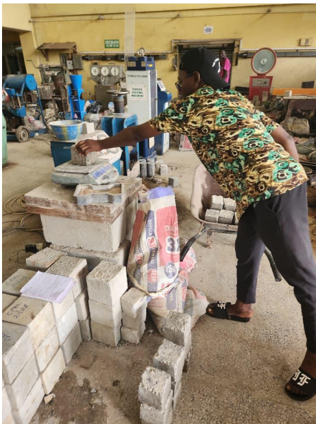
Plate A3: Weighing of Cubes for Mass Determination
