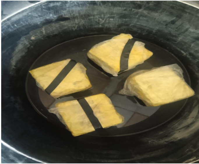
Plate A4: Sorptivity Test Setup and Sealing of Cube Faces
