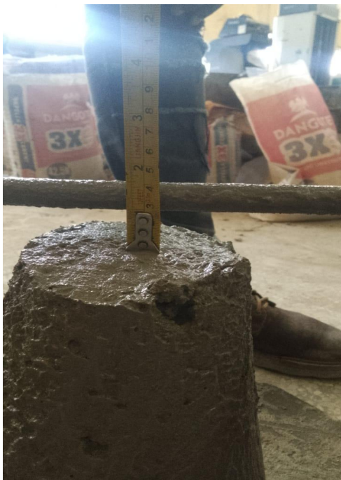
Plate A1: Slump Test Setup
