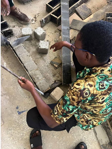
Plate A2: demolding of dried concrete cubes
