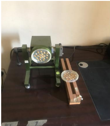
Plate 4: maize seeds subjected to clinorotation in a simulated microgravity environment using a clinostat and maize seeds subjected to normal gravity
