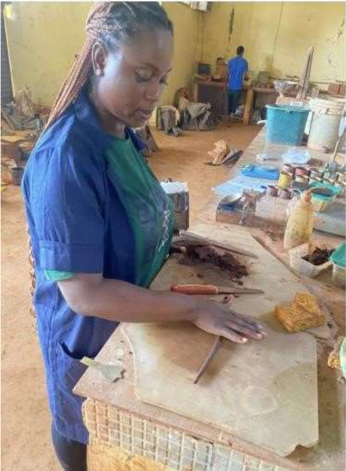
PLASTIC LIMIT TEST IN PROGRESS
