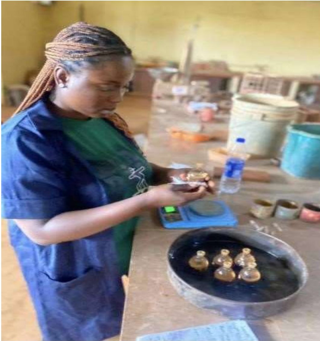
SPECIFIC GRAVITY TEST IN PROGRESS
