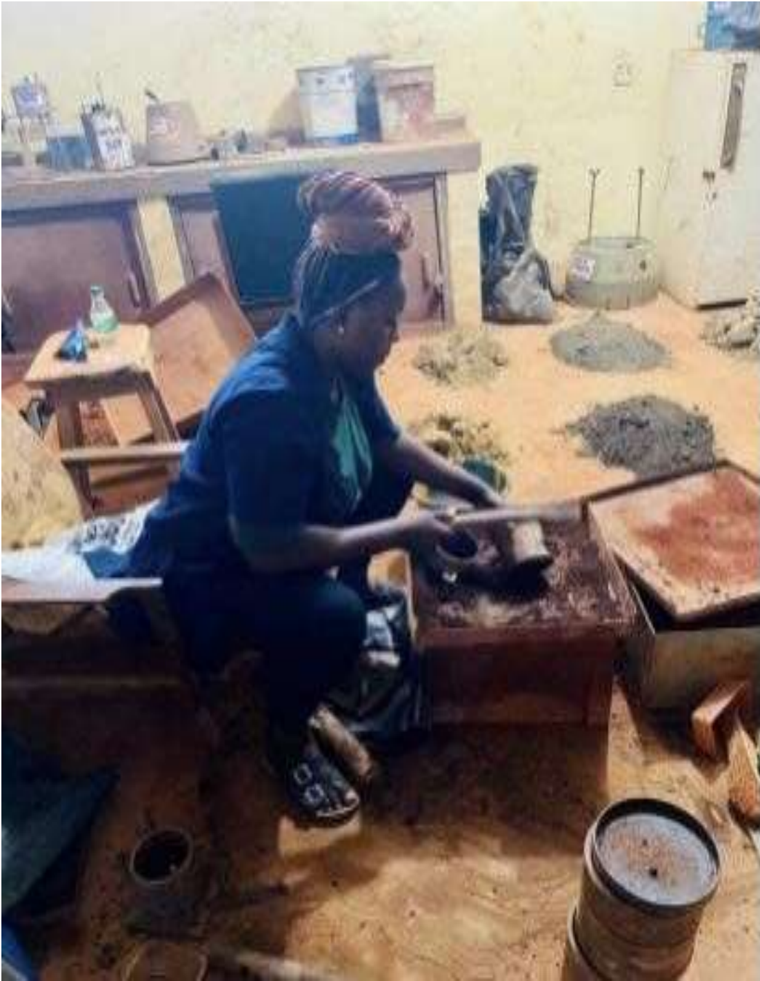
COMPACTION TEST IN PROGRESS
