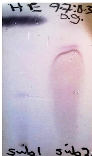
Figure 3.12: Chromatogram showing the preparative TLC fractions SF 1 G and SF 2 G of O. gratissimum oil obtained from F1 (CF 1 G). Adsorbent- Silica gel GF 254 , Solvent system: C 6 H 14 -CH 3 COOC 2 H 5 (9.7:0.3). Spray reagent: 12% H 2 SO 4
