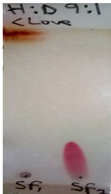
Figure 3.15: Chromatogram showing preparative TLC fractions SF 1 E and SF 2 E of E. caryophyllus oil obtained from F1 (CF 1 E). Adsorbent- Silica gel GF 254 , Solvent system: C 6 H 14 -CH 2 Cl 2 (9:1). Spray reagent: 12% H 2 SO 4
