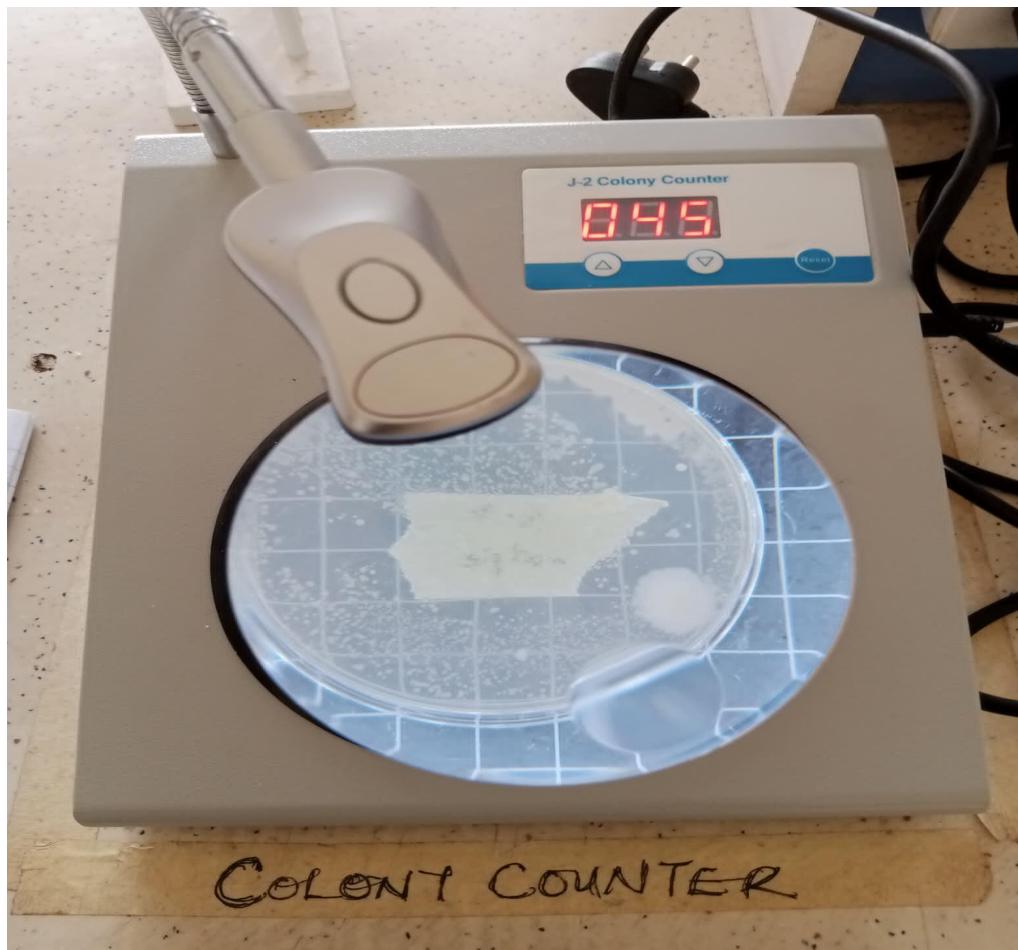
Plate 4: A colony counter and petri dish containing microorganisms in Nutrient Agar.
