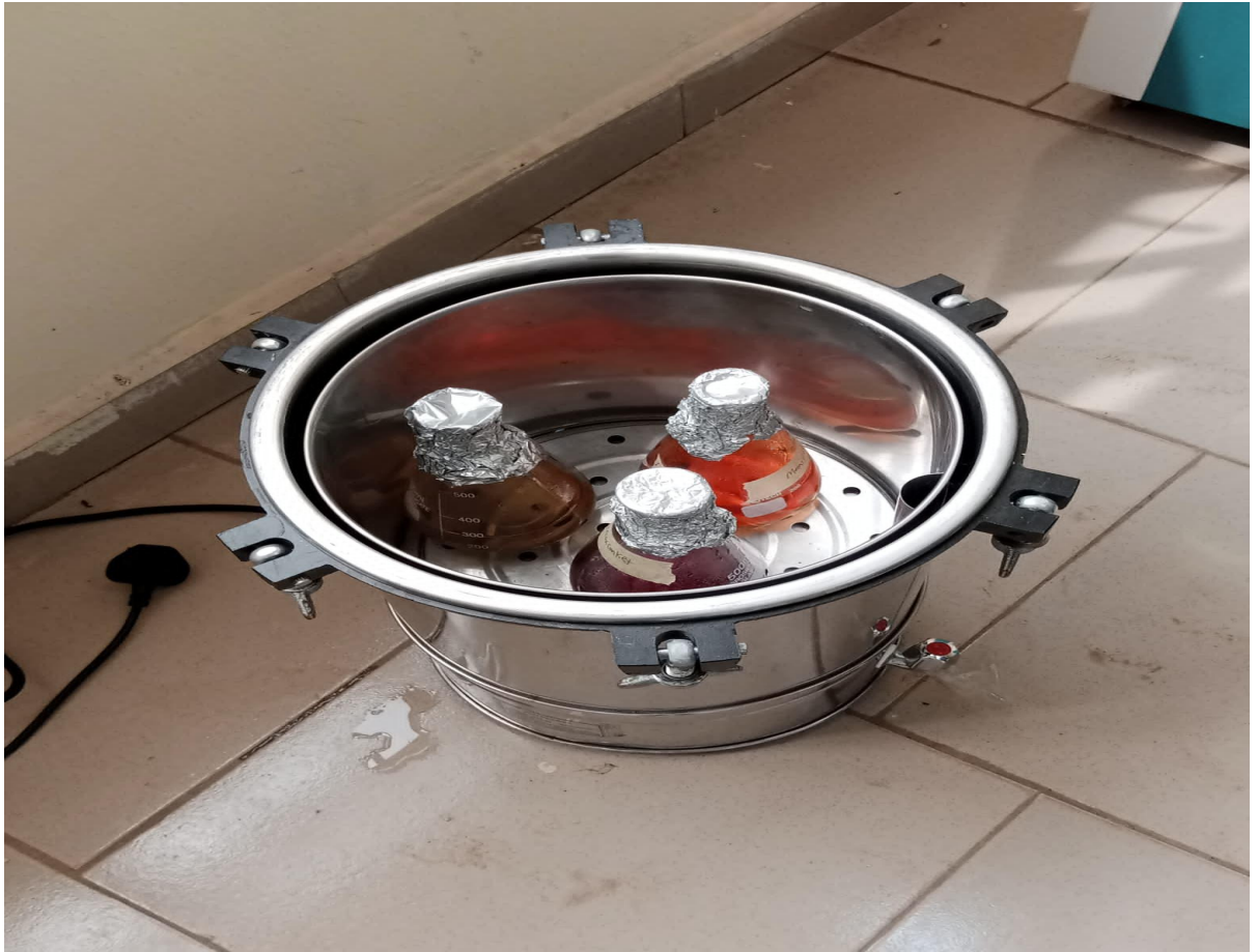
Plate 3: Culture media sterilized in the Autoclave at 121°C for 15 minutes at 15 psi
