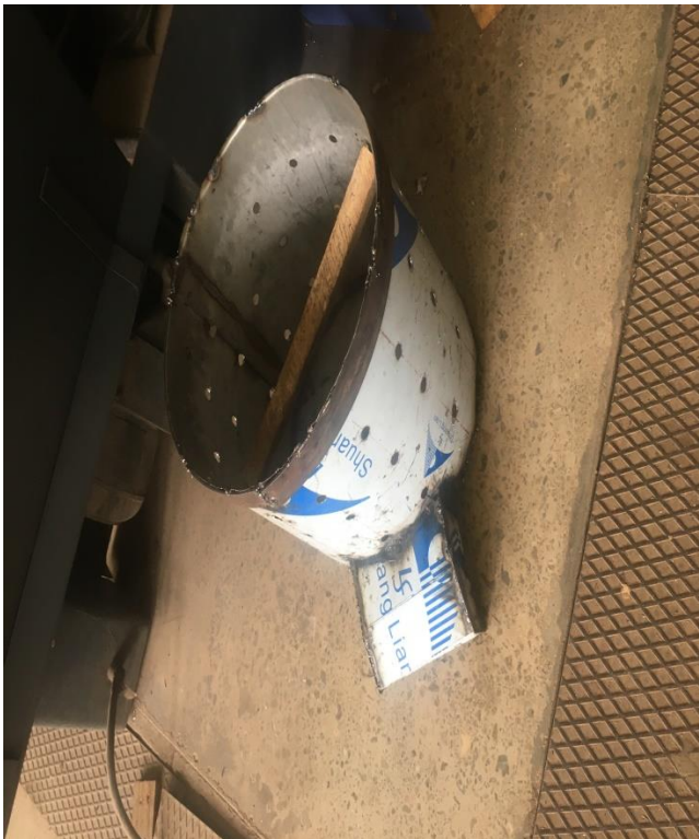
Holes drilled for the Rubber Fingers
