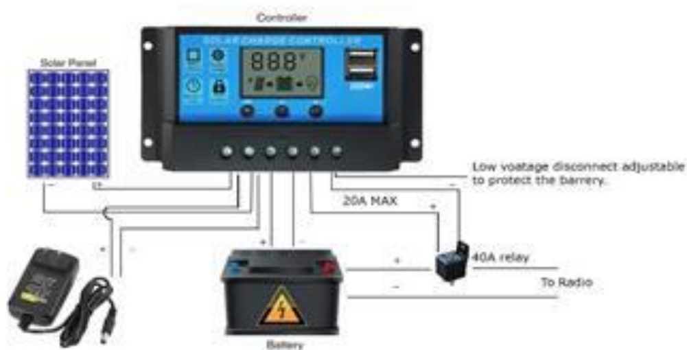
Figure 2.14: A charge controller connected to a solar panel
