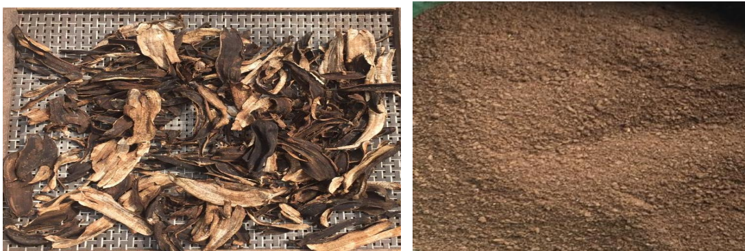
Figure 3.5: Plantain peels before and after grinding
