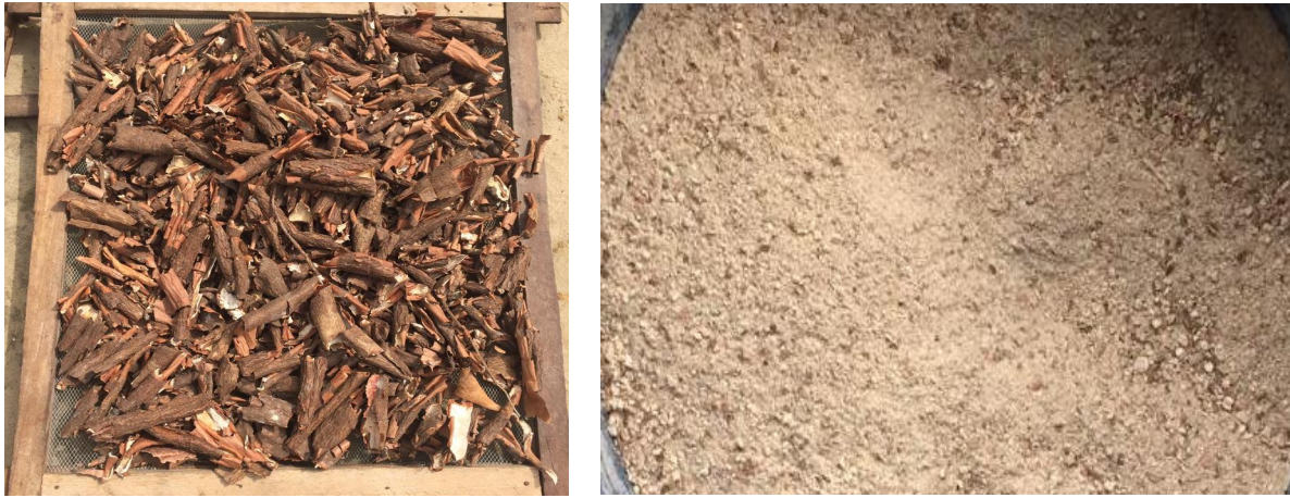
Figure 3.4: Cassava peels before and after grinding
