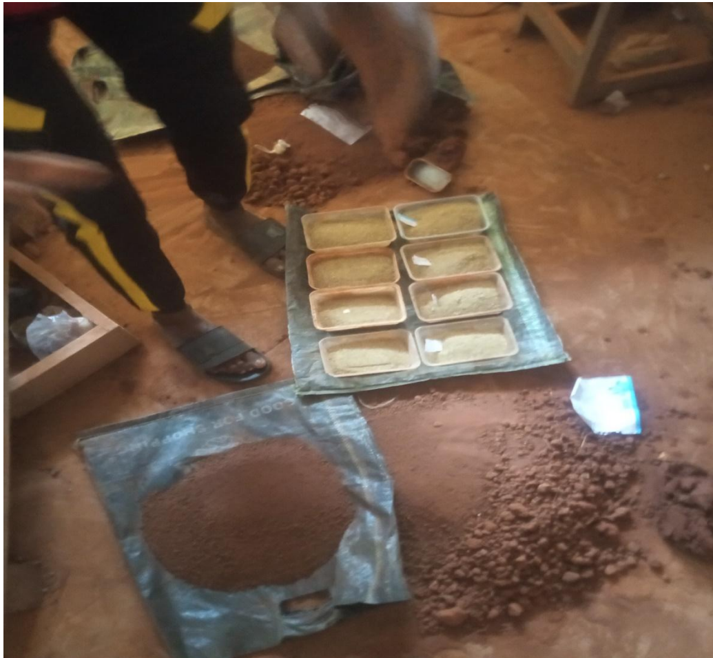
Figure 3: Raw laterite sample 1 and 2 , with orange peel stabilizer, at 2,4,6 and 8% for both samples
