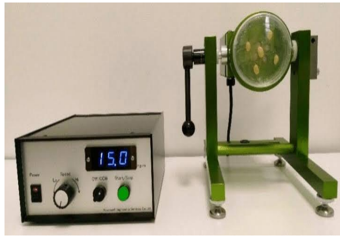
Figure 1: A clinostat used to stimulate a micro-gravity environment
