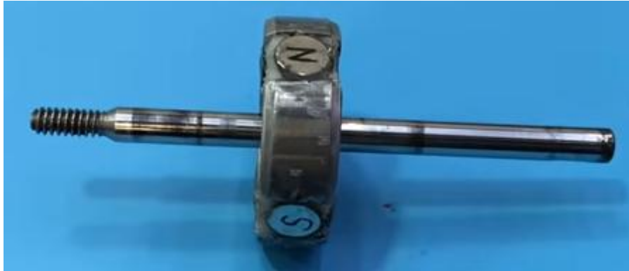
Figure 3.5: Attaching magnets to the rotor
