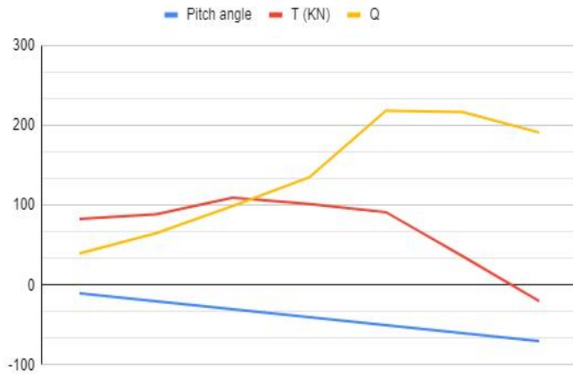
Figure 4.16: Graph showing trend for thrust and torque for negative increase in pitch angle
