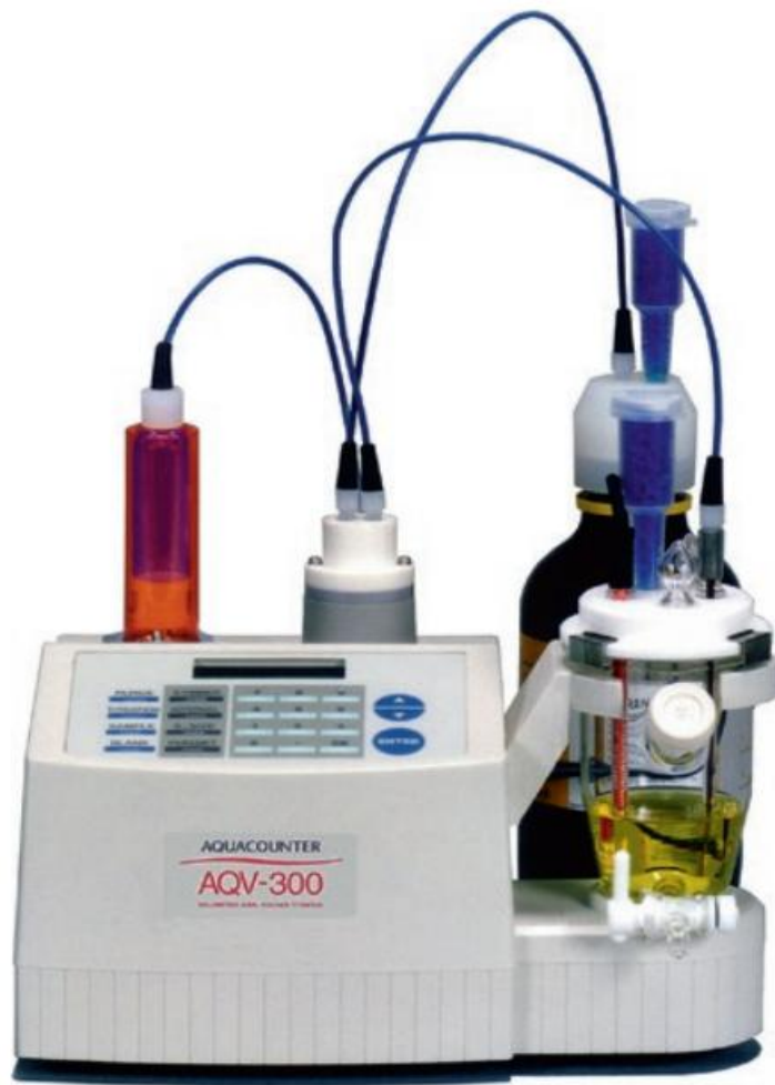
Fig 2.1. Automated Karl Fischer volumetric titration unit. (Source: Mauer and Bradley Jr, 2017).
