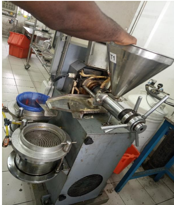
Plate. 2: Screw Press Mechanical Extractor
