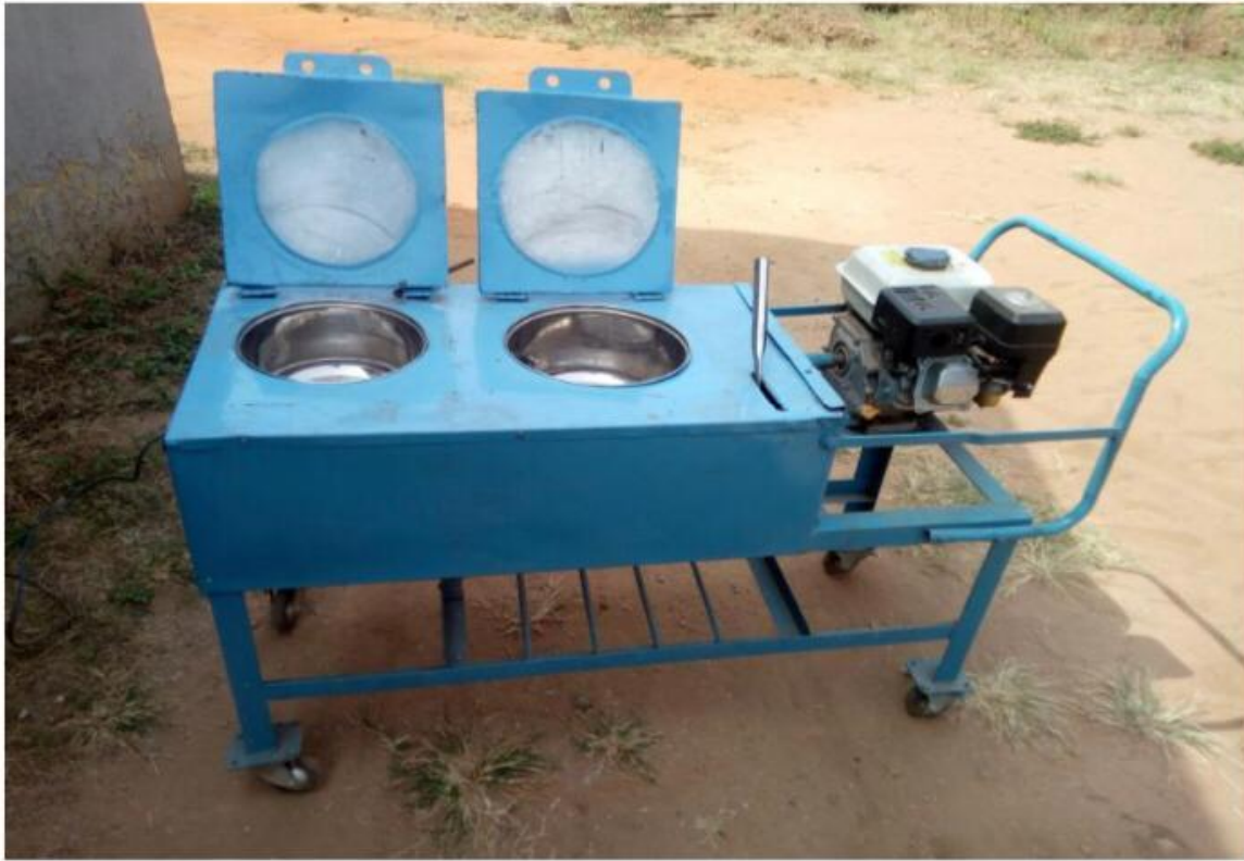
Figure 2.12: Developed pounding machine with chambers open
