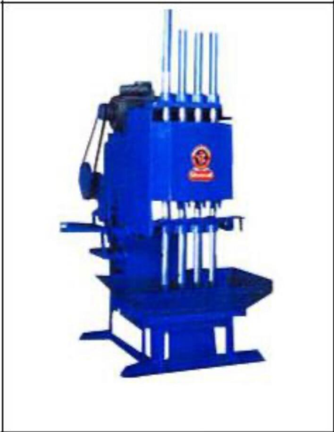
Figure 2.3 A pounding machine using a level system
