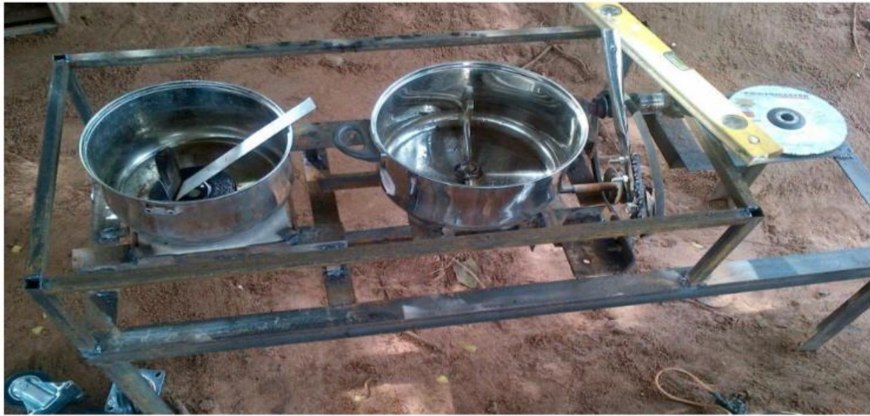
Plate 1 Fabrication process of yam pounding machine
