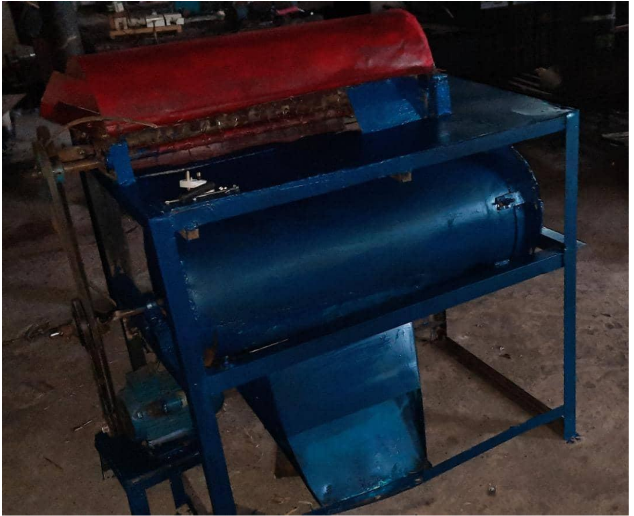
Fig 3.9b Final Assembly of Machine Showing the Maize Grain Outlet
