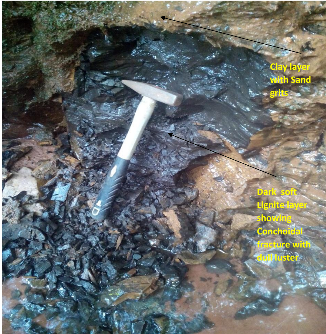
PLATE 3.1a; Rock exposure of Azagba-Ogwash Lignite (Yellow layer shows layers of Clay gritted with sands; Dark layers shows Lignite Layers 3m thick with Conchoidal fracture and dull lustre)
