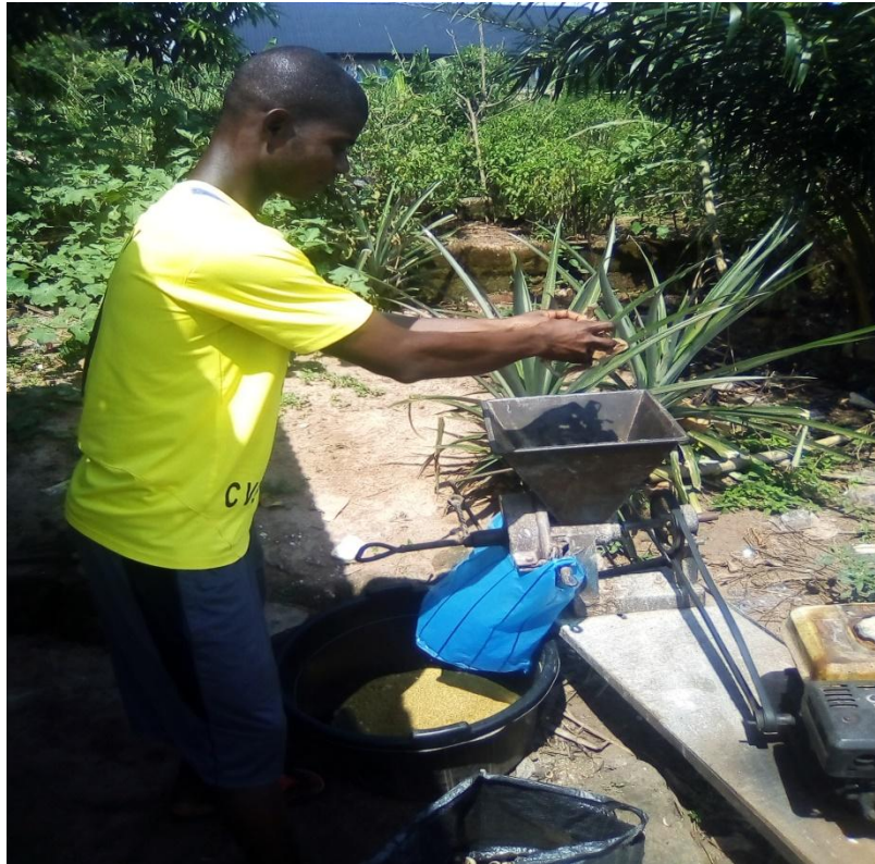
Figure 2(c) Grinding of the orange peels with a locally made engine.
