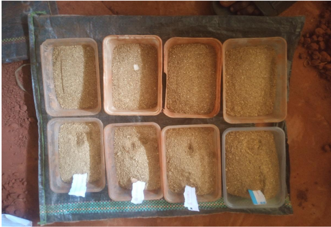
Figure 8: Raw laterite sample 1 and 2, with orange peel stabilizer, for CBR.
