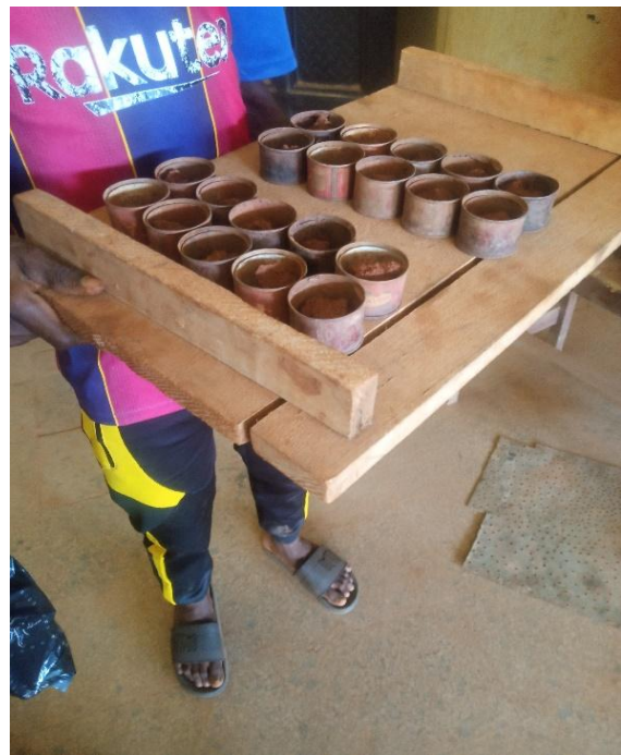
Figure 7: sample for oven-drying
