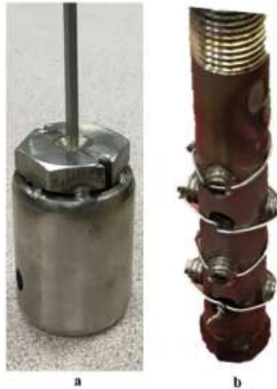
Figure 3.4 Top spider: a) Initial version b) Final version
