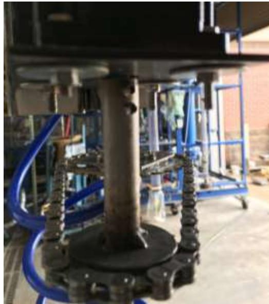
Figure 3.9 Stepper Motor with Azimuth Control Mechanism (Akita et al., 2020)
