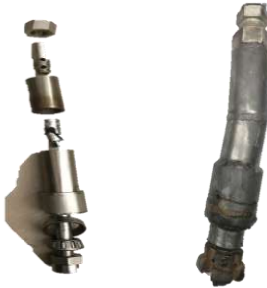
Figure 3.6 Bent sub and bit assembly: a) interior; and b) exterior
