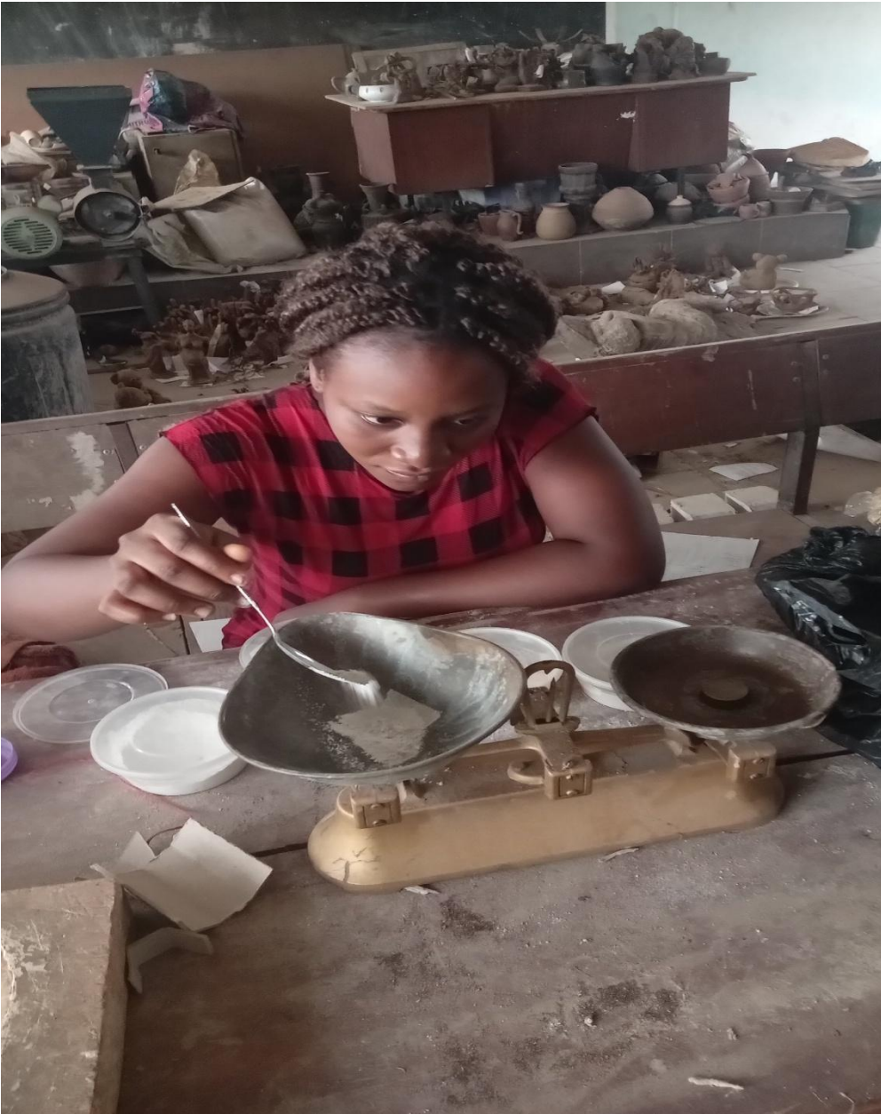
Figure 1 Weighing of the oxide (whitening) on the scale Photograph by Owolabi Emmanuel
