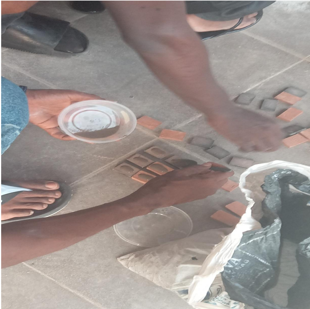
FIGURE 3 Application of the oxides on the test tiles Photograph by Azubuiké Precious
