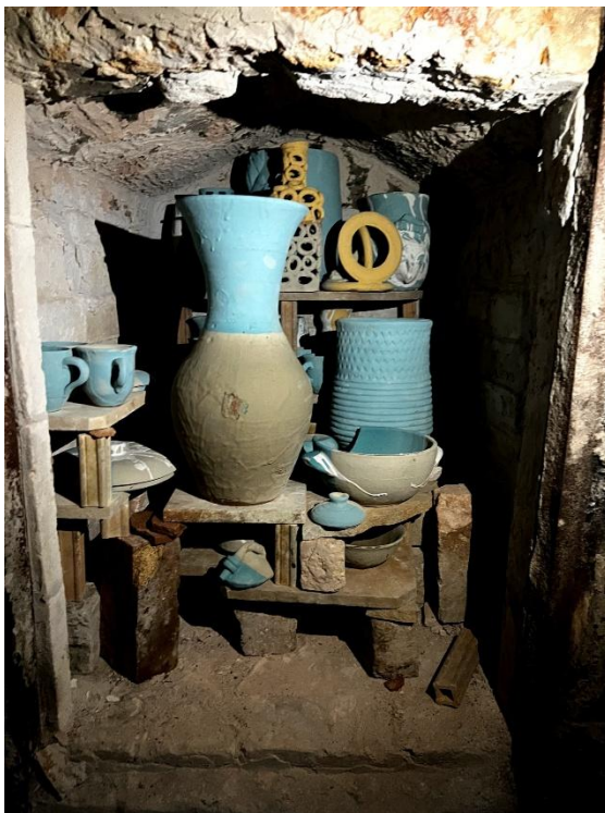
FIGURE 10 Arrangement of the ceramic wares in the kiln Photograph by Nnamani Felix
