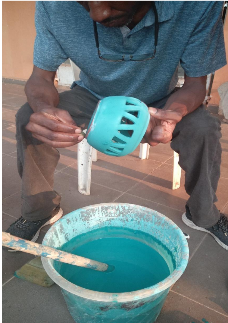
FIGURE 7 Dipping of a ceramic ware into the glaze Photograph by Azubuikie Precious
