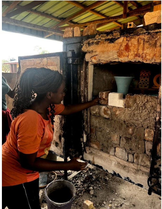
FIGURE 9 Adding of the bricks in the kiln Photograph by Nnamani Felix
