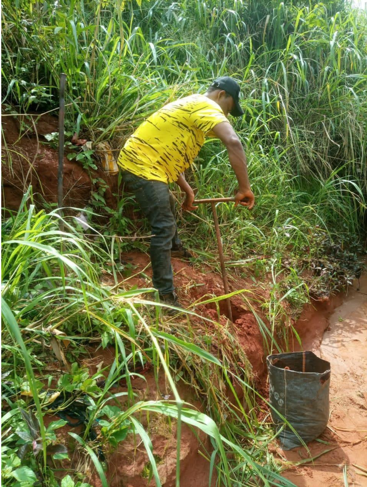
COLLECTION OF SOIL SAMPLE FROM SITE
