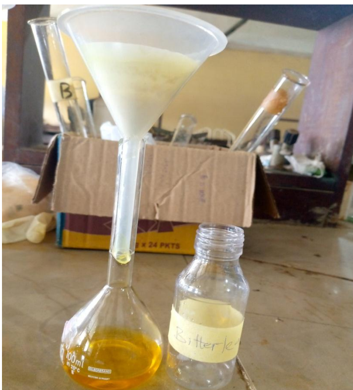
Figure 2.4: Filtration process of the digestate and 20ml distilled water for Bitter leaves sample.
