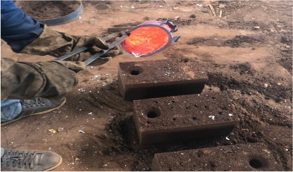
Fig 3.10 - Molten composite being poured into the cavity
