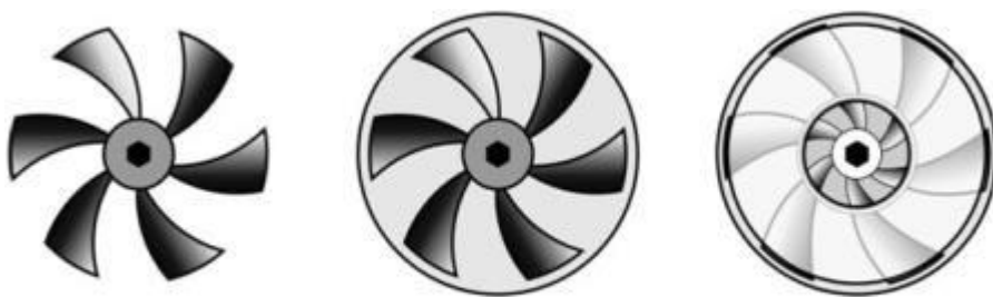
Fig 2.7 - Open, Semi Enclosed and Enclosed Impeller
