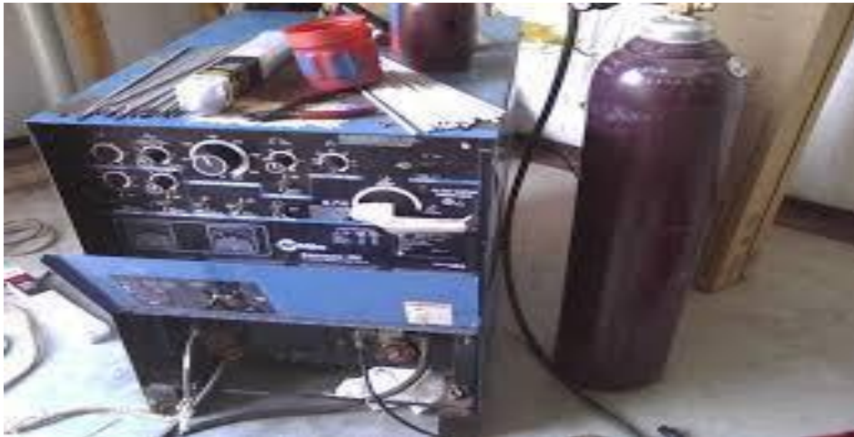
Plate 3.1: TIG welding machine with argon gas cylinder
