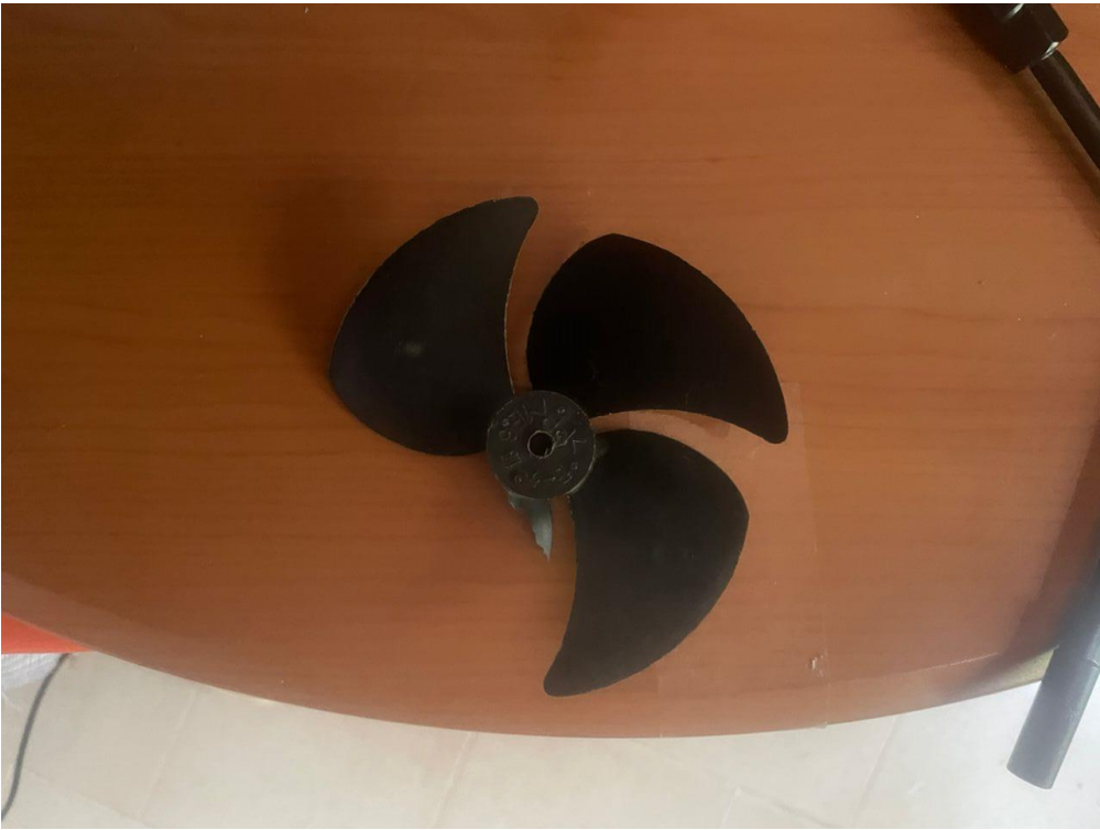
Figure 3.17 – Broken Plastic Fan blade from stress failure
